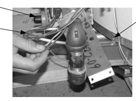
Burner Rack Mounting Screw
